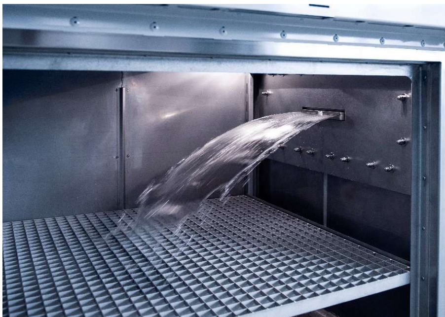
Splash water nozzle installed in the right side wall (installation of a 2nd nozzle possible)
